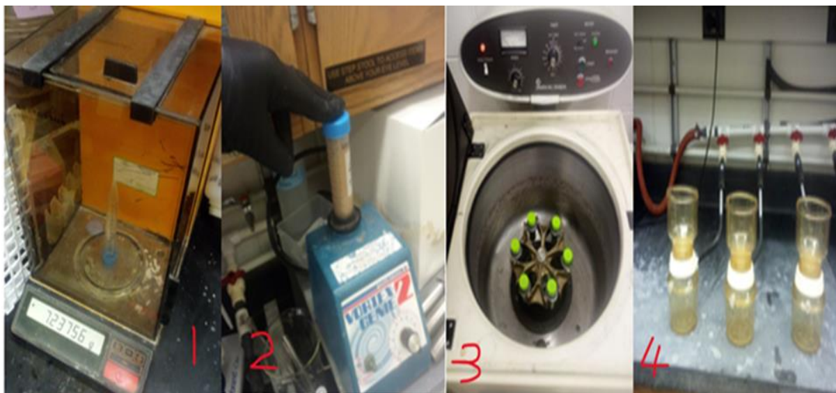
Figure 2.2: depicts the sequential steps of the experimental procedures of soil samples. (1) Weighing the soil samples using an analytical balance; (2) Mixing the samples with the help of a vortex mixer to guarantee homogeneity; (3) Centrifuging the samples to separate soil particles from the liquid phase; and (4) Filtering the samples with a vacuum filtration system to eliminate any leftover particulates in the extracted solution.
