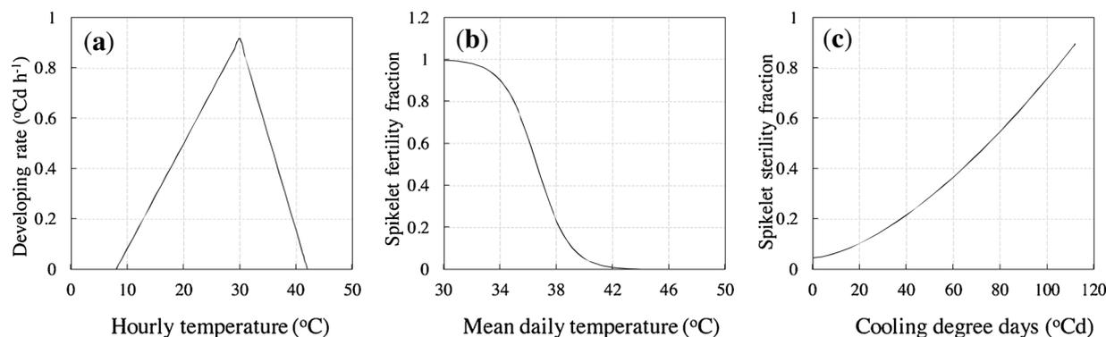
Fig. 2. The main response functions to simulate the direct and indirect effects of temperature increase on rice yield and irrigation. (a) Relationship between hourly temperature and developing rate. (b) Relationship between mean daily maximum temperature during the flowering period ( $0.96 < DVS < 1.22$ ) and spikelet fertility fraction. (c) The influence of cooling degree days on spikelet sterility fraction during booting and flowering periods ( $0.75 < DVS < 1.2$ ).
